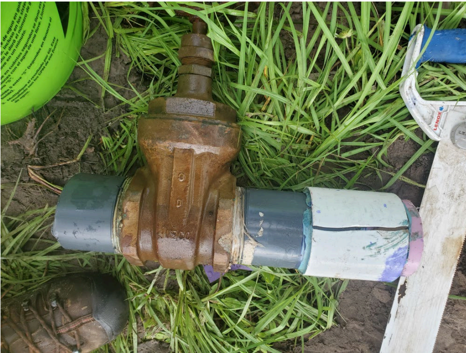
Cracked fitting on gate valve along north side of Covington Stone.
