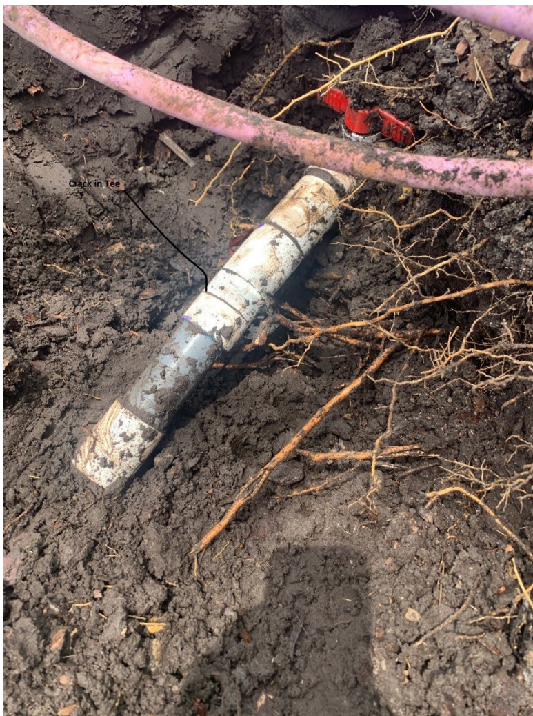
Cracked tee on mainline for N-controller.
